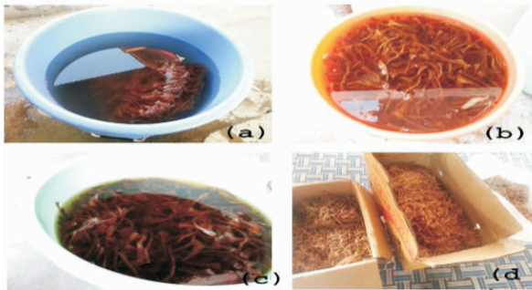
Figure 5(a) Jute soaked in NaOH (b) Jute soaked in Polymer (c) Jute in Distilled Water (d) Oven Dried Jute
