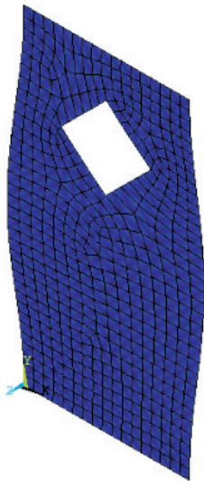
Figure 12. Fundamental Mode Shape of Plate with Rhombus Hole at Top
