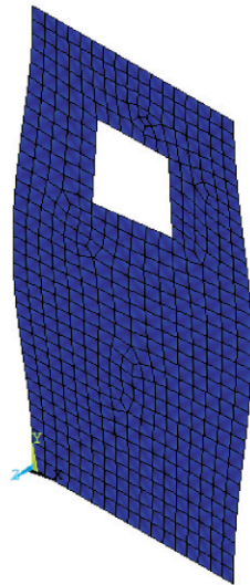
Figure 8. Fundamental Mode Shape of Plate with Square Hole at Top
