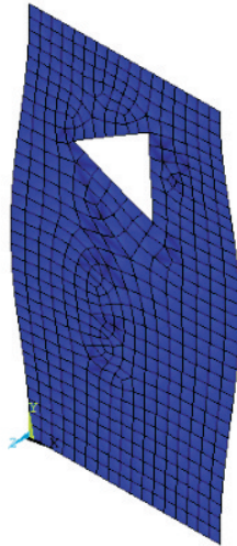
Figure 4. Fundamental Mode Shape of Plate with Triangular Hole at Top
