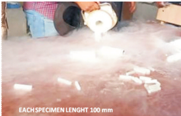
Figure 5. Cryogenic Treatment of Solution Treated Samples before ECAP
