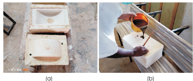
Figure 8. (a) POP Sink Mold (b) Pouring of Limestone-Clay Composite into Plaster Mold
