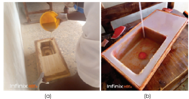
Figure 7. (a) Pouring Limestone Polyester Composite into Wooden Mold (b) Sink Cast
