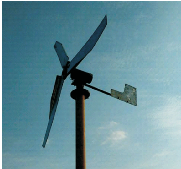
Figure 8. Aluminum Based Blades HAWT installed at Test Location
