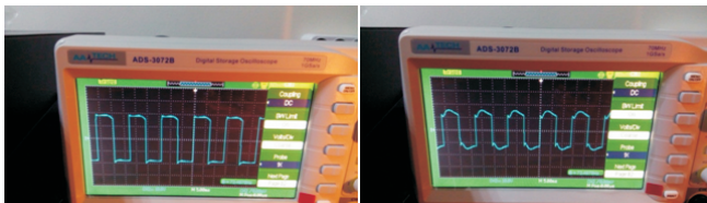
Figure 8. Observation of the Voltage Output Waveforms with Resistive and Inductive Load
