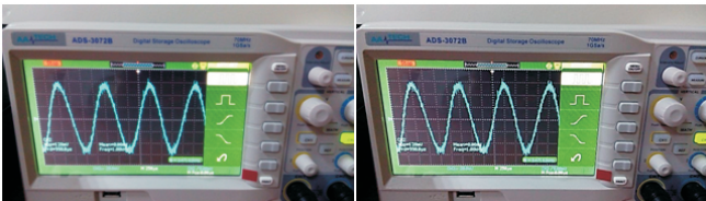
Figure 16. Observation of the Voltage Output Waveforms with Resistive and Inductive Load
