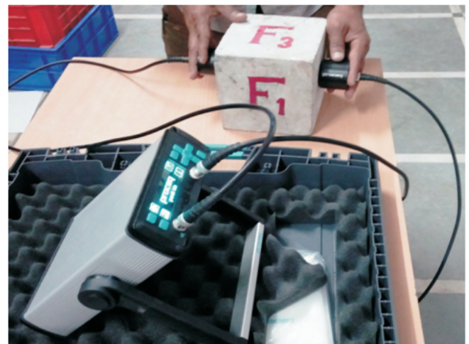
Figure 7. UPV Measurement on F 1 , F 2 and F 3 of a Cube Specimen
