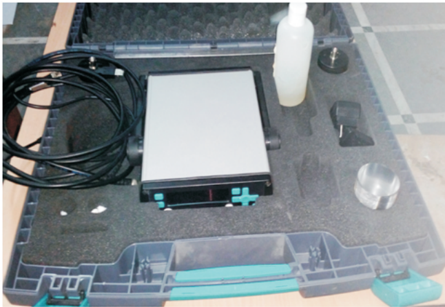
Figure 8. Ultrasonic Pulse Velocity Test apparatus
