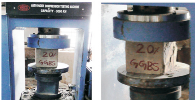
Figure 4. Compression Test on GRCCP Specimens
