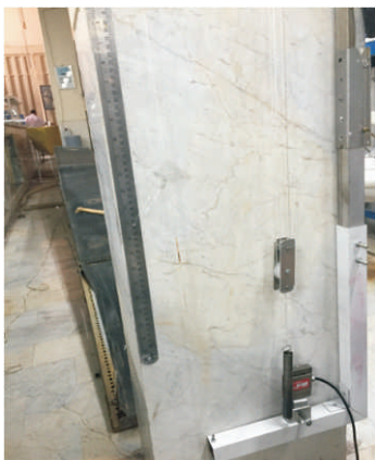
Figure 4. Spring Test for Determining the Stiffness
