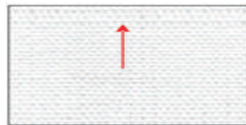
Figure 3. Irregular Pick Density
