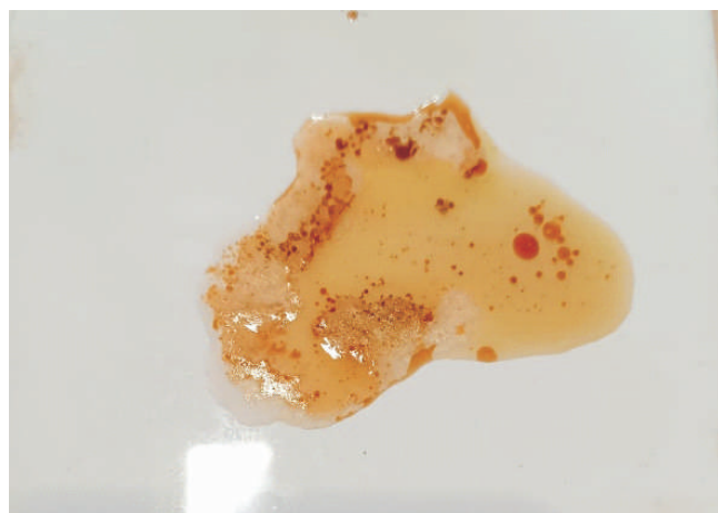
Figure 10. Functional Group Test for Type Base (aniline) on Ceramic Tile
