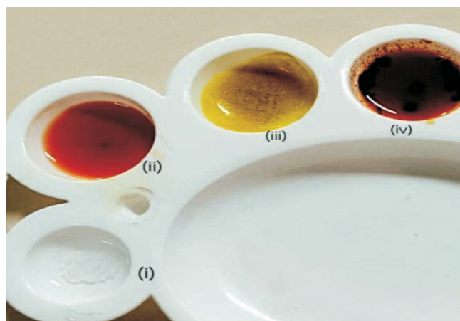
Figure 12. Functional Group Test for Different Types of Organic Compounds using Plastic Groove Plates
